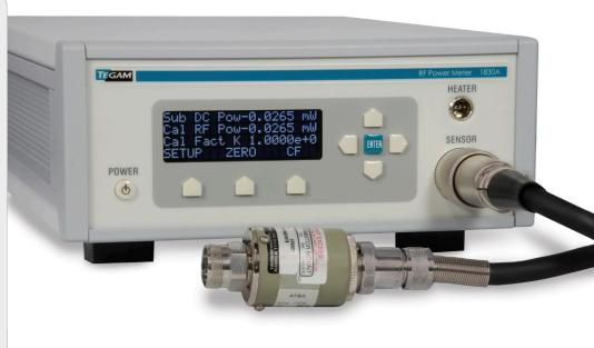
Thermistor RF power sensors are universally recognized as the most accurate means to measure and transfer RF power. The TEGAM Model 1830A was designed to operate with all types of thermistor RF power sensors while reducing uncertainties. It combines a modern DC substitution bridge with a precision measurement system to provide consistent, calibrated RF power readings manually or automatically.
