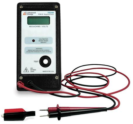
If the voltage sensed on the test leads exceeds approximately 1 V, the R1M-B will not take any additional readings. However if there is no voltage (or less than approximately 1 V) on the test leads, the instrument will automatically switch to the megohmmeter mode, whereupon the internal 500 V supply is connected to the test leads and the measured resistance is displayed.
